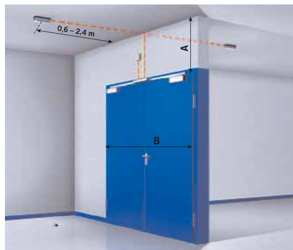
1 lintel-mounted detector and 2 ceiling-mounted detectors
